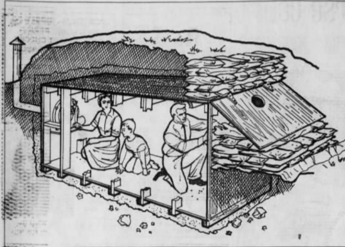
Outside semimounded plywood box shelter
